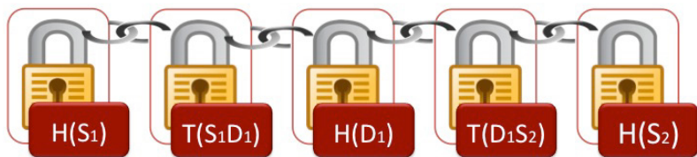
Figure 3: A Supply Chain Provenance. The figure illustrates a product transported from S1 to S2, and the corresponding proofs, which are being used to create a secure supply chain provenance.
